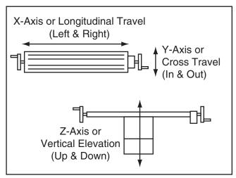
Figure 16. The directions of table movement.
